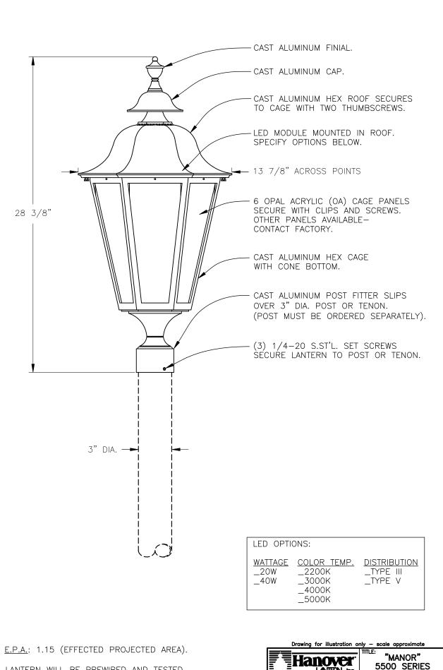
LANTERN WILL BE PREWIRED AND TESTED. ALL ELECTRICAL COMPONENTS ARE U.L. LISTED. ALL MOUNTING HARDWARE IS SUPPLIED.
